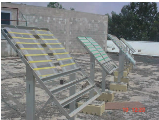
Figure 1. Experimental set up for exposing the polymer samples in natural weathering condition. [Color figure can be viewed in the online issue, which is available at wileyonlinelibrary.com .]
